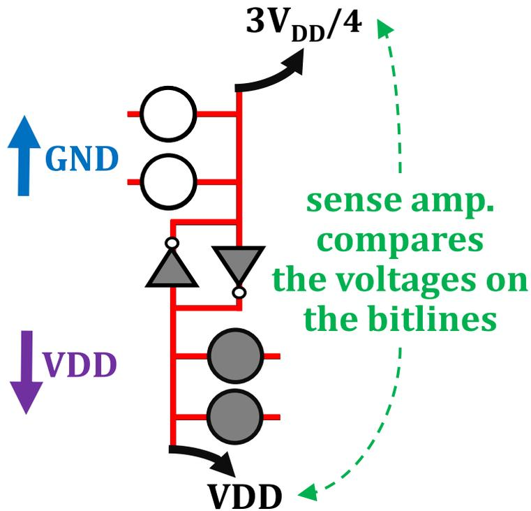
$V_{DD}=1$  &  $GND=0$
