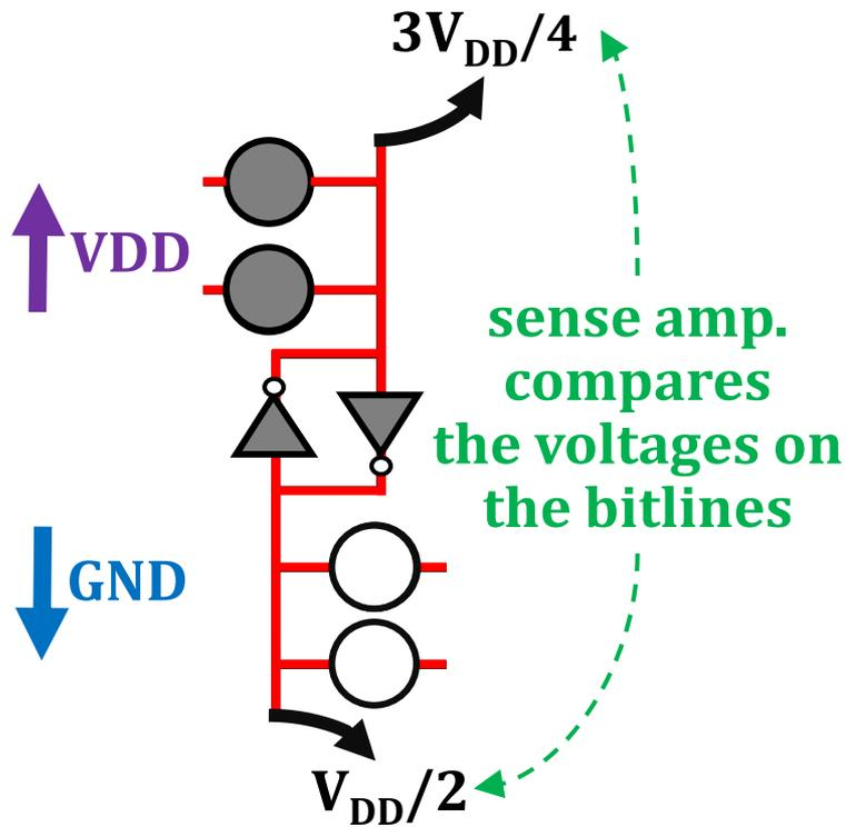
$V_{DD}=1$  &  $GND=0$
